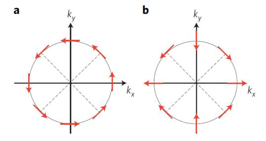
Spin texture due to Rashba (a) and linear (b) Dresselhaus SO coupling when strain is applied along [001].
