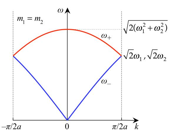
At the edges of the Brillouin zone the highest frequency  $\omega_{-}(\pi/2a)$  of the acoustic branch, however, coincides with the lowest frequency  $\omega_{+}(\pi/2a)$  of the optical branch.
