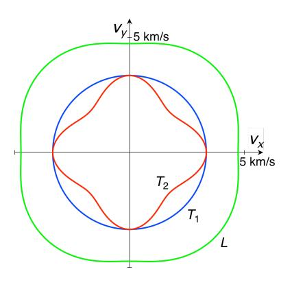
The isotropic and cubic elastic tensors are identical, except that for an isotropic solid  $c_{44}=\frac{1}{2}(c_{11}-c_{12})$ . An anisotropy parameter A is defined as
