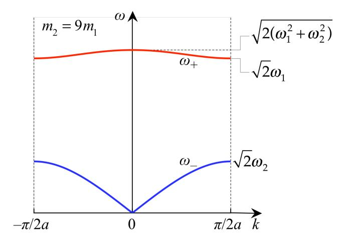
If the limit  $m_1 \ll m_2$  the density of normal modes  $g(\omega)$  of the optical branch can be approximated by a  $\delta$ -function.
