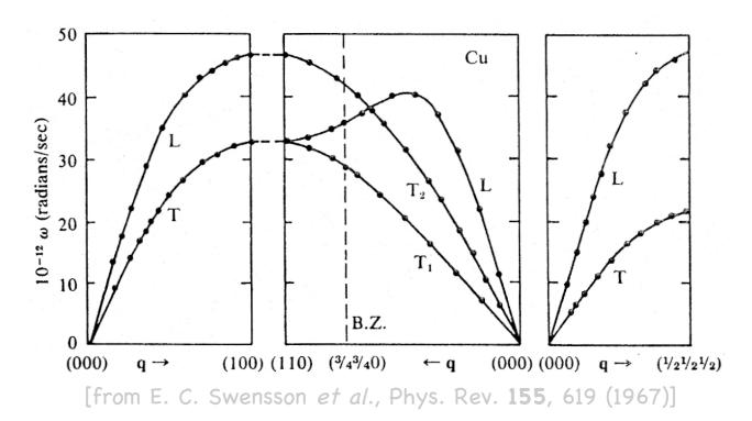
The wave vector is plotted in units  $ka/2\pi$ . Data points correspond to excitations with certain frequency  $\omega$  and wave vector k, i.e., to phonons. For some high-symmetry directions the transverse modes are degenerate.
