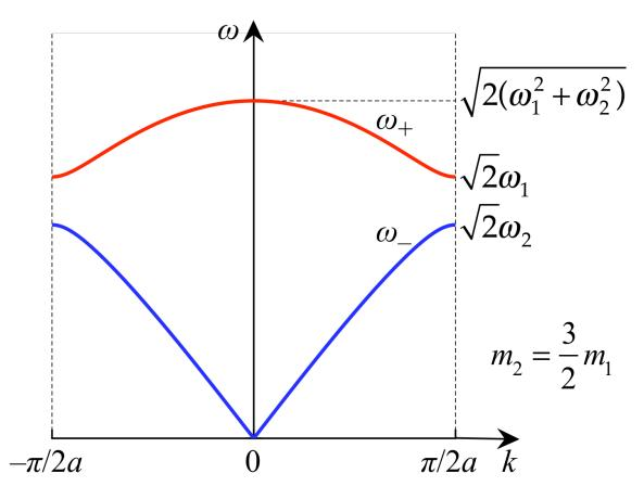
The width of a gap formed at  $k=\pi/2a$  is  $\Delta\omega=\sqrt{2}(\omega_1-\omega_2)$ .
