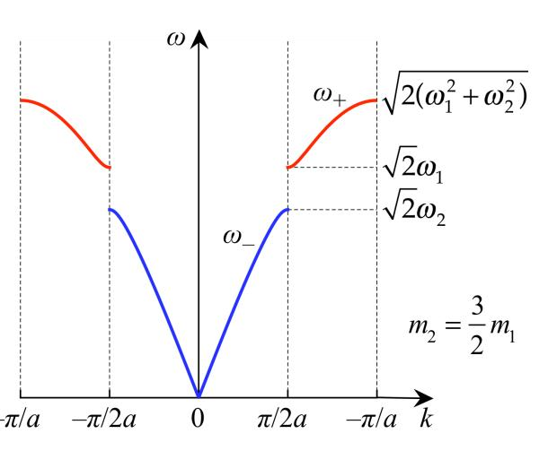
Optical branches appear in the excitation spectrum of the Bravais lattice with the basis that contain two or more atoms. An optical branch appears even when a diatomic basis contains two identical atoms.
