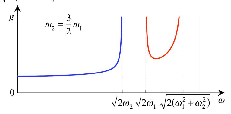
If the limit  $m_1\ll m_2$ , the frequency of the optical branch  $\omega_+$  weakly depends on k, the group velocity  $\partial\omega/\partial k$  is small, and the width of the optical branch is  $\Delta\omega_+\approx\omega_+(0)m_1/2m_2$ .
