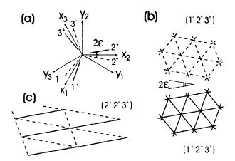
FIG. 2. Domain walls (a) EQT (b), and ELT (c) textures in quartz.
