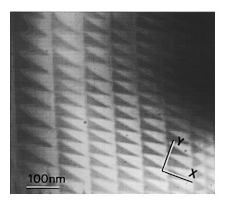
FIG. 1. Dark field image (TEM, Bragg spot (110)) of the ELT phase.
