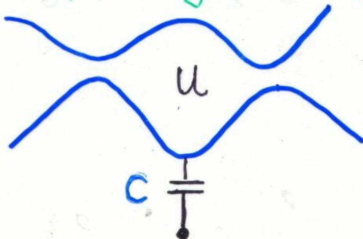
$$S_{II}(\omega) = \omega^2 S_{QQ}(\omega) = \omega^2 C^2 S_{UU}(\omega) \\ = 2\omega^2 C_\mu^2 (R_q kT + R_v |eV|)$$
