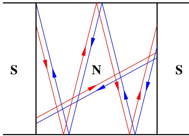
Chaotic dynamics: low-energy Andreev states in a dirty SNS junction are completely suppressed by interference. Density of states acquire a minigap.
