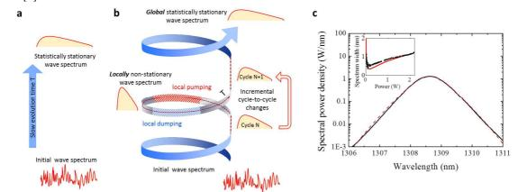
Fig. 1. Wave kinetics in active cyclic systems. (a) Classical wave kinetics. (b) Wave kinetics of active cyclic systems. (c) Measured (black line) and calculated within nonlinear kinetic theory (red line) generation spectrum of random fiber laser. At insert: spectrum broadening over generation power in experiment (black) and theory (red).
